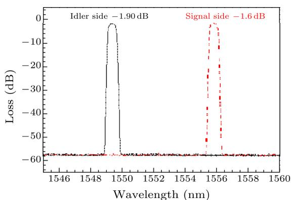
**Fig. 2.** The transmission spectra of the filtering and splitting system. Dashed line: signal side; solid line: idler side.
