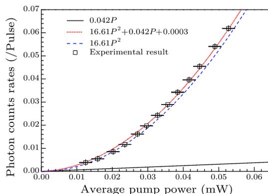
**Fig. 3.** The photon-count rate at the idler side under different pump levels. Square dots: experimental data; dotted line: fitting curve of experimental data; dashed line: contribution of the CPPs; solid line: contribution of the SpRS and residual pump.
