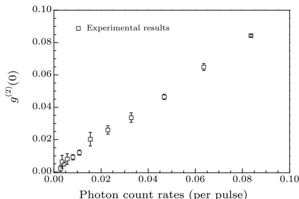
Fig. 5. The measured  $g^{(2)}(0)$  of the HSPS versus idler-side photon-count rate.
