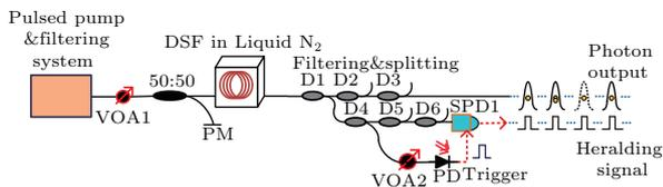
**Fig. 1.** Experimental setup of the fiber-based HSPS at 1.5  $\mu\text{m}$ . VOA: variable optical attenuator; PM: power meter; PD: photo detector; DSF: dispersion-shifted fiber; SPD: single-photon detector; D1~D6: DWDMs.
