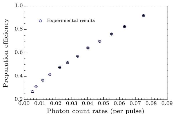
Fig. 4. The measured preparation efficiency of the HSPS versus idler-side photon-count rate.
