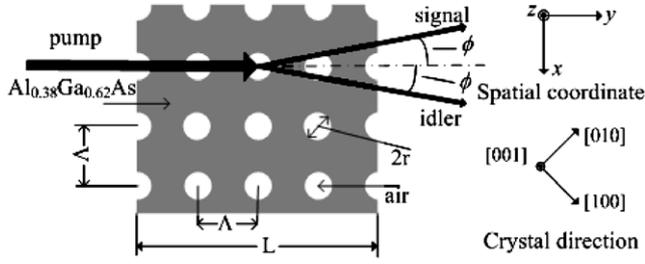
Fig. 1. Top view of the 2-D PC geometry with square lattices of  $\text{Al}_{0.38}\text{Ga}_{0.62}\text{As}/\text{air}$ .
