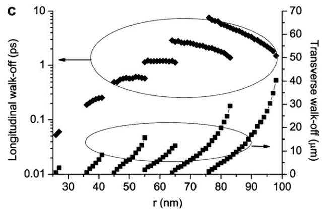
Fig. 3. (a) Phase-matching condition versus period  $\Lambda$  and hole radius  $r$  of 2-D PC. (b)  $\phi^H$  (triangle) and  $\phi^V$  (circle) versus  $r$  under different  $\Lambda$ . (c) Longitudinal (diamond) and transverse (square) walk-offs versus  $r$  under different  $\Lambda$  for a 2-D PC with  $L = 3$  mm.  $\Lambda$  are equal to 140 nm, 160 nm, 180 nm, 200 nm, 220 nm, 240 nm for the lines from the left to the right in (b) and (c).
