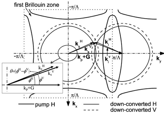
Fig. 2. Sketch of equi-frequency contours of the H pump wave and the down-converted H and V waves ( $\Lambda = 200$  nm and  $r = 65$  nm are selected for clarity). The magnified part shows the relation between the angles of the wave vectors.
